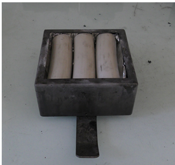
Figure 2. Sample holder with cables D28 for cone calorimeter test.
