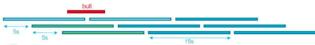
Figure 3: Audio segmentation with overlapping. In this example, the first four segments are labeled as bull .
