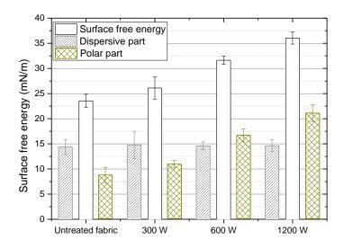
**Figure 5.** Evolution of the free surface energy of the polyester textile with the evolution of the polar and dispersive parts.
