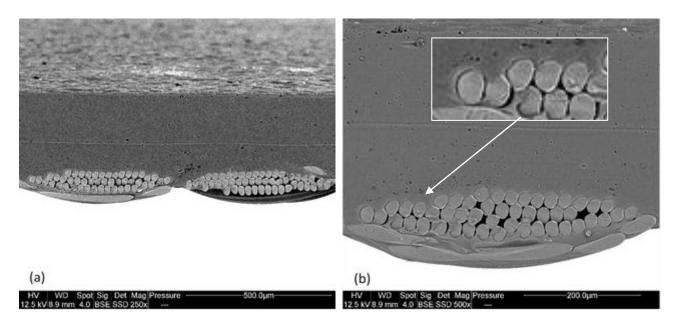
**Figure 2.** Final structure of the textile (SEM image – 2a. magnification x 250 and 2b. magnification x 500)).
