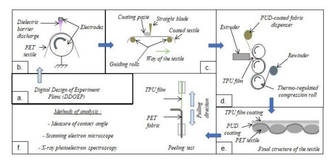
**Figure 1.** Method of processing and characterization; a. Digital Design of Experiment plans used for plasma parameters screening; b. Atmospheric pressure DBD treatment in ambient air of the PET textile; c. Coating of the PUD paste onto the textile, followed by an over drying step; d. TPU film deposited by an extrusion-cast technique; e. Final structure of the textile; f. Characterization methods used, details of the peeling test are given.
