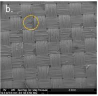
**Figure 4.** SEM observations of the PET textile after peeling. View of the textile after the peeling of the coating (a. without plasma treatment and b. with plasma treatment).
