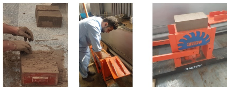
Figure 6. Production of earthen elements: from left to right, sun-dried brick, CEB, CEB extruded from the mould.
