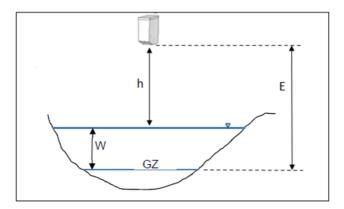
Fig. 3. Water level measurement technique by stream radar (modified from Sommer, 2014). To retrieve water depth (W), the distance (E) between the sensor and a reference level corresponding to the mean of the channel bottom elevation (GZ) is entered into the sensor so that the sensor can automatically determine W from the difference between E and the measured h.
