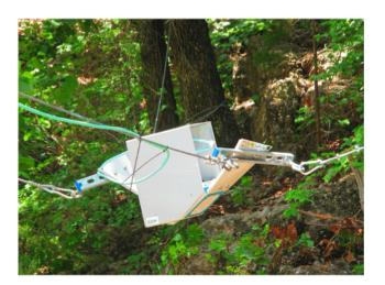
Fig. 9. Photographs of the Falls Creek, Oklahoma, stream radar following the 17 May 2017 flash flooding event.
