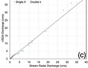
Fig. 7. Scatter plots of discharge (in  $m^3$  s<sup>-1</sup>, or cms) as measured by a conventional station and the stream radars using the single- and double- $k_g$  optimization schemes at (a) Mill Creek, (b) Cherry Creek, and (c) Walnut Gulch.
