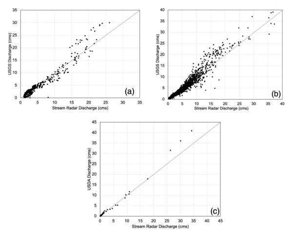
Fig. 5. Scatter plots of discharge (in  $m^3$  s<sup>-1</sup>, or cms) as measured by a conventional station and the stream radars at (a) Mill Creek, (b) Cherry Creek, and (c) Walnut Gulch using a default  $k_g$  coefficient of 0.85.
