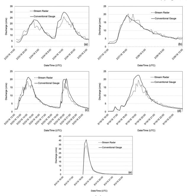
Fig. 6. Hydrographs of radar-measured and conventional discharge estimates (in  $m^3$  s<sup>-1</sup>, or cms) for flooding events at (a, b) Mill Creek, (c, d) Cherry Creek, and (e) Walnut Gulch using a default  $k_g$  coefficient of 0.85.
