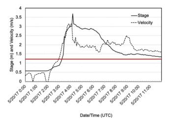
**Fig. 8.** Hydrographs of radar-measured stage (solid) and surface velocity (dashed) for a flash flooding event at the Falls Creek site near Davis, Oklahoma. The initial alert thresholds for both stage and velocity that was used for this event is shown in red. (For interpretation of the references to colour in this figure legend, the reader is referred to the web version of this article.)
