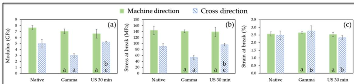
**Figure 11.** Bending tests results for (a) modulus; (b) stress at break; (c) strain at break ; Gamma column: If value is different compared to Native ( $p$  value < 0.05) letter b; otherwise letter a; US 30 min column: If value is different compared to Native, letter b otherwise letter a. In addition, if value is different compared to Gamma, letter c, otherwise left blank.
