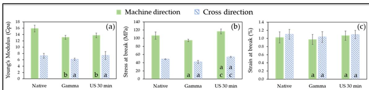
**Figure 10.** Tensile test results for (a) Young's modulus; (b) stress at break; (c) strain at break; Gamma column: If value is different compared to Native ( $p$  value < 0.05), letter b; otherwise letter a; US 30 min column: If value is different compared to Native, letter b otherwise letter a and if value is different compared to Gamma, letter c, otherwise left blank.
