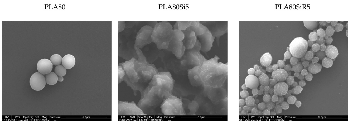
Figure 10. SEM micrographs of the PA11 nodules after extraction of PLA with chloroform for PLA80, PLA80Si5, and PLA80SiR5.
