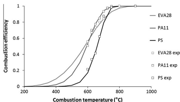
Fig. 15. Modeling curves and experimental data for PA11, PS, and EVA28.
