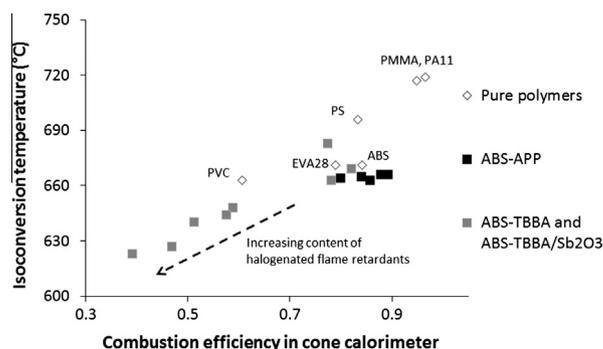
Fig. 20. Isoconversion temperature versus combustion efficiency in the cone calorimeter (irradiance 50 kW/m<sup>2</sup>) for flame retarded ABS and pure polymers.
