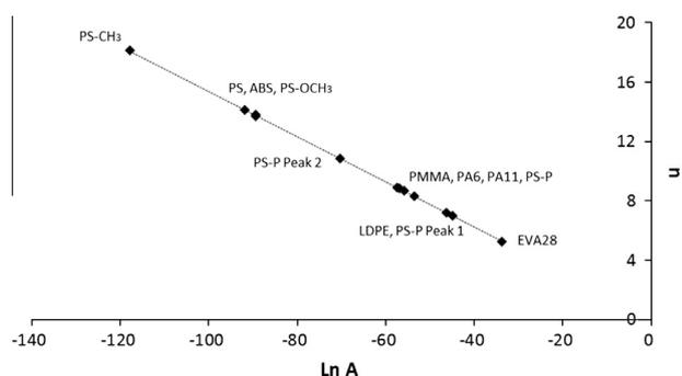
Fig. 14.  $n = f(\ln A)$  for the polymers under consideration.
