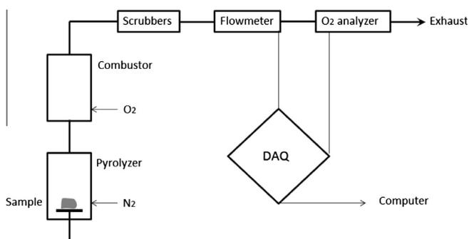
Fig. 1. Schema of pyrolysis-combustion flow calorimeter (from [9]).
