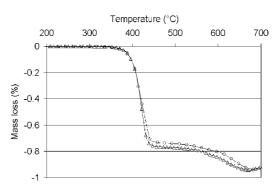
Fig. 8. TGA curves in air (5 °C/mn) of PET filled with 3% red P+2% Alumina in function of the specific surface area of alumina, ( $\bigcirc$ )Al<sub>2</sub>O<sub>3</sub> sBET = 250 m<sup>2</sup>/g, ( $\triangle$ ) Al<sub>2</sub>O<sub>3</sub> sBET = 130 m<sup>2</sup>/g.
