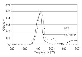
Fig. 3. Gram Schmidt curves of unfilled PET and PET with 5% red phosphorus as a function of temperature.
