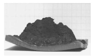
Fig. 12. Optical micrograph showing the intumescence for 3% red P+6% glass fibres +2% Al<sub>2</sub>O<sub>3</sub> in PET.
