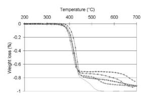
Fig. 2. TGA curves of filled and unfilled PET in air and argon (5 °C/ min). (—) PET in air, ( $\Delta$ ) PET in Argon, ([]) 3% red P, (\*) 5% red P, ( $\bigcirc$ ) 3% red P+2% Al<sub>2</sub>O<sub>3</sub>.
