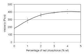
Fig. 4. Shear viscosity of PET as a function of the percentage of red phosphorus.
