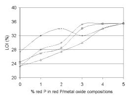
Fig. 6. Limiting oxygen index (LOI) of PET as a function of the red P/ metal oxide composition. ( $\Box$ ) red P/Al<sub>2</sub>O<sub>3</sub>, ( $\bigcirc$ ) red P/MgO, (\*) red P/ Fe<sub>2</sub>O<sub>3</sub>, ( $\triangle$ ) red P.
