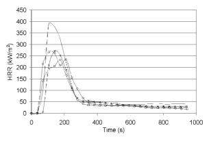
Fig. 5. Heat Release Rate of filled and unfilled PET as a function of time. (—) PET, ([]) 3% red P, (\*) 5% red P, ( $\bigcirc$ ) 3% red P+2% Al<sub>2</sub>O<sub>3</sub>.
