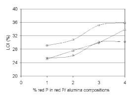
Fig. 7. Influence of the median diameter and specific surface area of alumina on the Limiting Oxygen Index of filled PET for several red P/ alumina compositions. ( $\triangle$ ) red P, alumina (ATH calcinated at 700 °C) median diameter 2.5 µm, sBET = 130 m<sup>2</sup>/g, synthetic alumina median diameter 0.5 µm, sBET = 5.6 m<sup>2</sup>/g.
