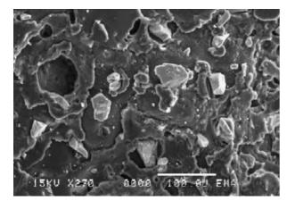
Fig. 1. SEM micrograph ( $\times$ 270) of broken cross sections of filled PET (5% red P).
