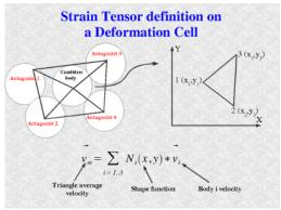
Fig. I.1 : Deformation cell definition
