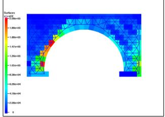
Fig. III.9 : The spherical component of the stress tensor at t = 5 seconds
