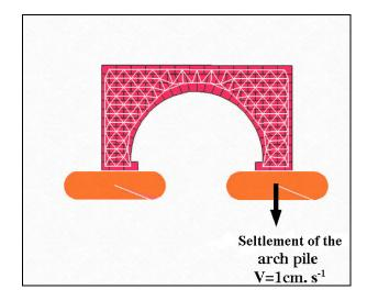
Fig. III.6 : Arch geometry and solicitation definition
