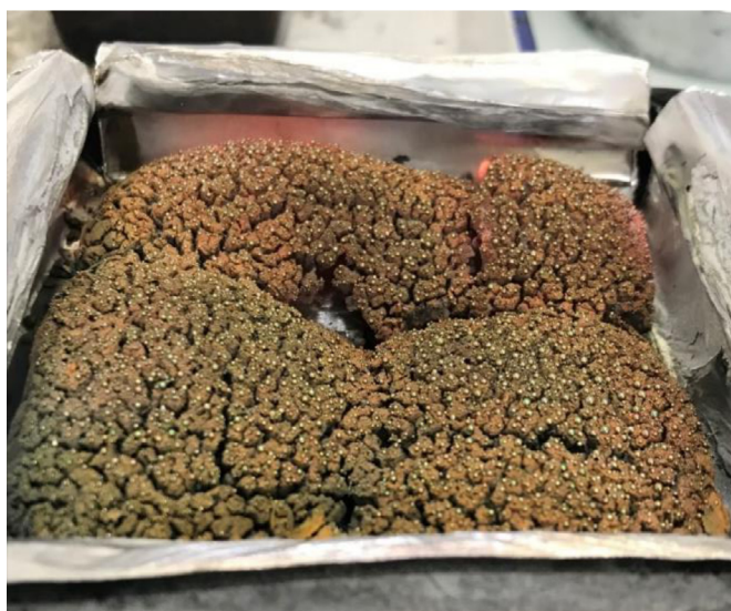
Fig. 16. Kyowaglas residue covered with leaded beads after a cone test.
