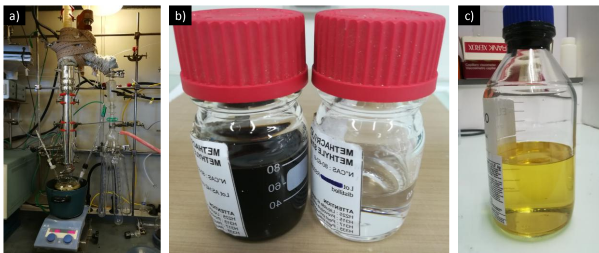
Figure 4: (a) Used vacuum distillation setup, (b) distillation input liquid (dark) and distillate (transparent) and (c) Recycled Elium 188-O (rElium) resin obtained from polymerisation of recycled MMA
