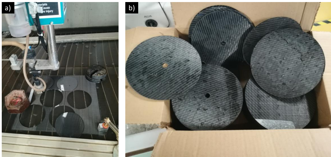
Figure 1: Water jet cutting machine (a) and discs cut with the desired diameter (b)
