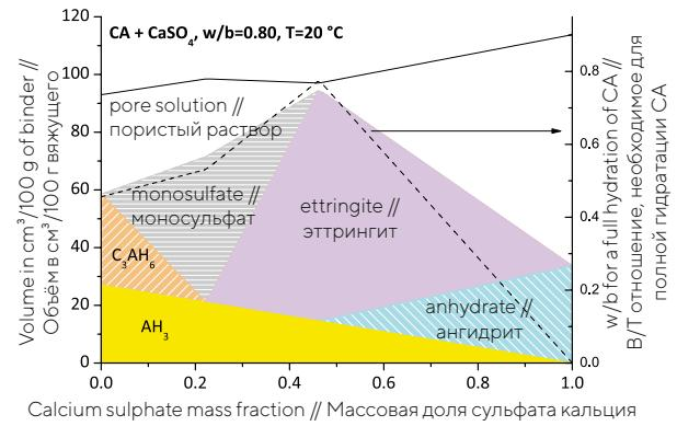
Fig. 6. Thermodynamic phase assemblage modelling of the hydration of CA blended with calcium sulphate as a function of calcium sulphate mass fraction in the unhydrated blended cement at  $w/b = 0.80$ . Volume expressed as  $\text{cm}^3/100 \text{ г}$  unhydrated blended cement (left-hand side). Minimum  $w/b$  ratio required for complete hydration of CA is shown on the right-hand axis, adapted from [33]
