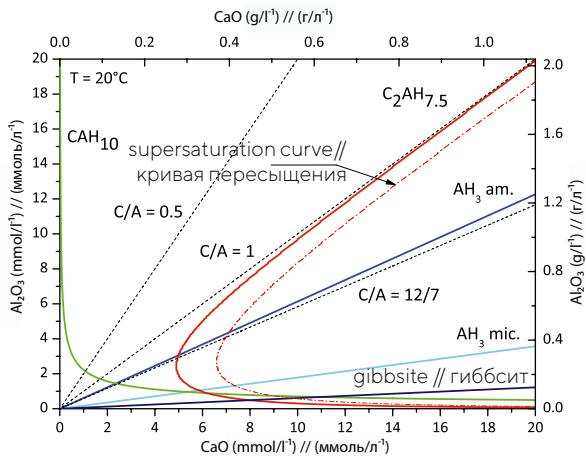
Fig. 3. C-A-H solubility diagram at  $T = 20^\circ\text{C}$  as a function of the  $\text{C}/\text{A}$  ratio in the unhydrated CAC. Thermodynamic data were taken from the PSI-GEMS and CEMDATA 14.01 databases. Supersaturation curve of  $\text{C}_2\text{AH}_8$  is calculated according to the equation proposed in [12]
