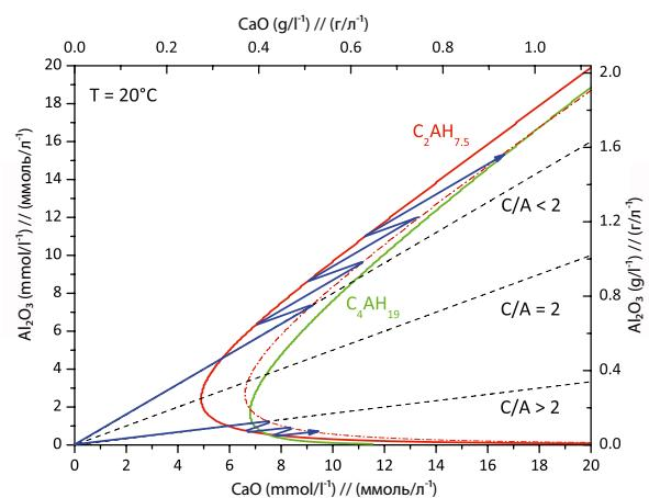
Fig. 4. Diagram explaining the variation of the composition of the solution with time in the case of the dissolution of a phase with  $\text{C}/\text{A} < 2$  (for example  $\text{C}_{12}\text{A}_7$ ) and of a phase with  $\text{C}/\text{A} > 2$  (for example  $\text{C}_3\text{A}$ ), adapted from [14].
