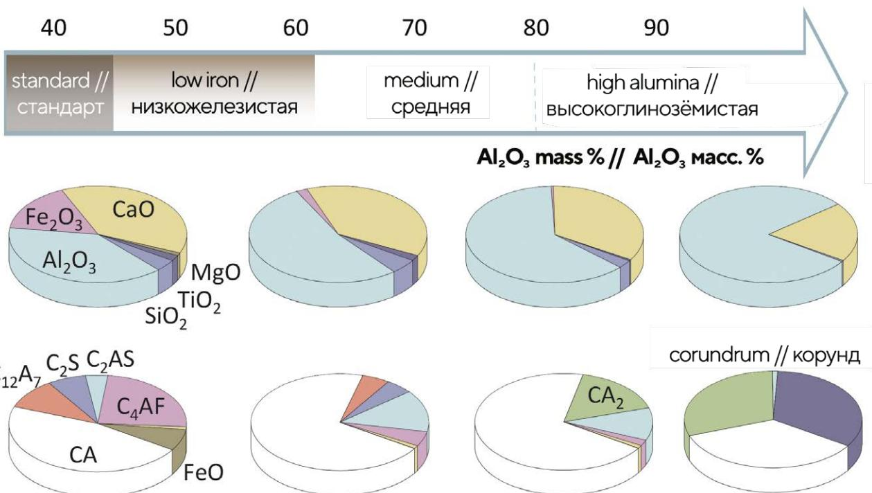
Fig. 2. Chemical composition and mineralogy of calcium aluminate cements
