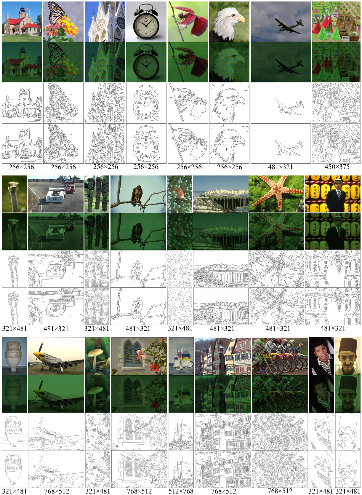
Fig. 2: Additional Results (arranged in rows): binary images are calculated by Rosin method (see original paper). From top to bottom: Original Full-Color Image, Bayer CFA Image, Edge detected by SESCDE, Edge detected by SSCDE. BE CAREFUL: compressed files.
