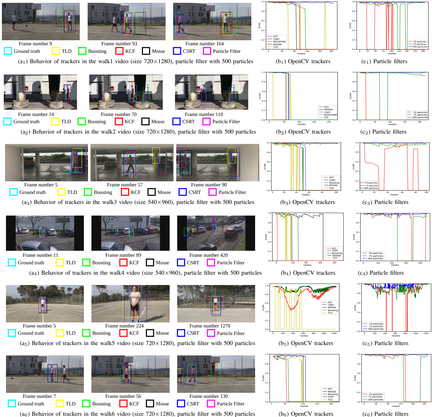
Fig. 4. Comparison of particle filter and tested OpenCV trackers on videos containing human(s) acquired with a moving camera.
