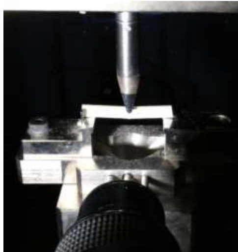
Figure 2 : Close up of sample and impactor, showing macro lens in front
