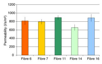
Fig. 6. Fibre permeability
