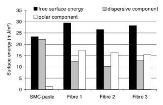
Fig. 2. Influence of the sizing amount applied onto the fibre surface on the surface energy of the glass fibres.
