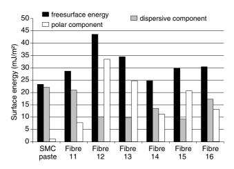
Fig. 5. Influence of the polyester nature on the surface energy of the glass fibres.
