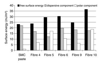
Fig. 4. Influence of the deposit method of the antistatic agent on the surface energy of the glass fibres.
