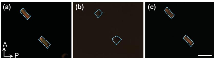
**Figure 6.** Micrographs of pillars (E-VC4 ( $n = 3$ ), 10% crosslinker) observed at different temperatures. The pillars were cut off from the structured surfaces and suspended in silicone oil to observe the shape change with temperature under polarizing optical microscope. The pillars were heated at a) 30 °C, b) 96 °C, and then cooled back to c) 48 °C. The dotted lines outline the shape of the pillars to guide the eye. Scale bar: 100  $\mu\text{m}$ . A: Analyzer; P: Polarizer.
