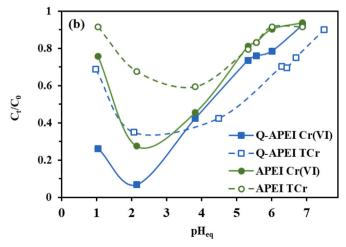
**Fig. 1.** Effect of pH on the Cr(VI) and TCr sorption using APEI and Q-APEI:  $q_{\rm eq}$  (a) and  $C_t/C_0$  (b) ( $C_0$ : 100 mg Cr(VI)  $L^{-1}$ ; sorbent dosage: 0.5 g  $L^{-1}$ ; contact time: 48 h; shaking speed: 200 rpm; T: 20  $\pm$  1  $^{\circ}$ C).
