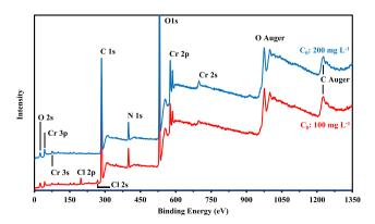
Fig. 6. HRES XPS survey of Q-APEI beads after Cr(VI) sorption at two metal concentrations (i.e., 100~mg Cr  $L^{-1}$  and 200~mg Cr  $L^{-1}$ ).
