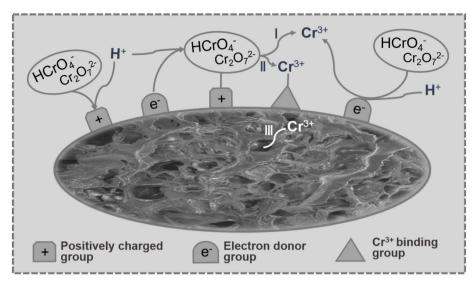
Fig. 7. Proposed mechanism of Cr(VI) sorption by Q-APEI beads.
