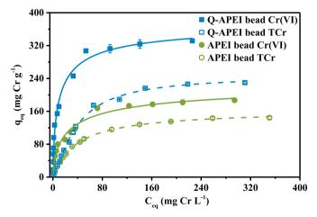
**Fig. 2.** Sorption isotherms of Cr(VI) and TCr using APEI and Q-APEI ( $C_0$ : 100 mg L $^{-1}$ ; sorbent dosage: 0.5 g L $^{-1}$ ; pH: 2; contact time: 48 h; shaking speed: 200 rpm; T: 20  $\pm$  1 °C. Lines (full lines-Cr(VI), dash lines-TCr) represent the modeling of sorption isotherms with the Sips equation and the parameters summarized in Table S3).
