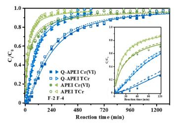
**Fig. 4.** Breakthrough curves of Cr(VI) and TCr sorption using APEI and Q-APEI in fixed-bed single path system ( $C_0$ : 100 mg L $^{-1}$ ; F (flow rate): 2 or 4 mL min $^{-1}$ ; sorbent mass: 0.5 g; volume: 1 L; pH: 2; T: 20  $\pm$  1 °C. Lines (full lines-Cr(VI), dash lines-TCr) represent the modeling with the Yan equation using parameters from Table S8).
