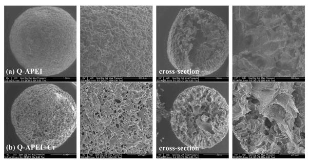
Fig. 5. SEM micrographs of surface and corresponding cross-section of Q-APEI beads before and after Cr(VI) sorption at pH 2 (magnification power: ×50 and × 250).
