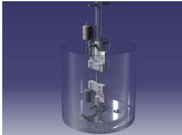
*Figure 3 – Set-up for environmental creep tests*
