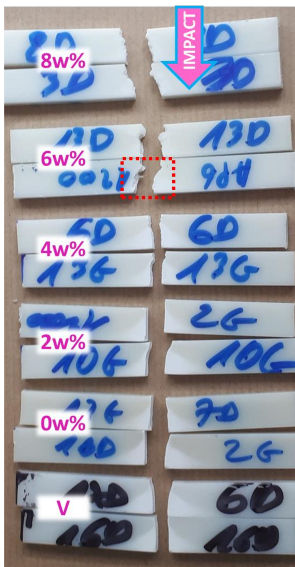
Figure 3. Picture of unnotched Charpy impact broken specimens of ABS gradually contaminated with PP—arrow shows direction of impact; rectangle points out dephasing at macro-scale.
