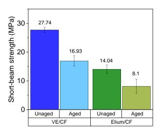
Figure 13: Short beam strength properties obtained by ILSS test for both aged and unaged CF /  $Elium^{TM}$  and CF / VE specimens
