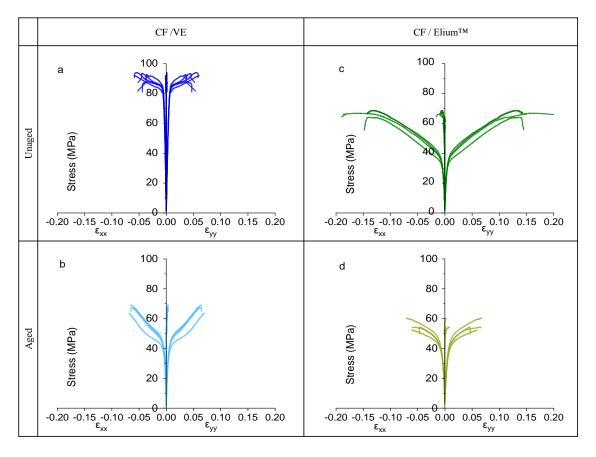
Figure 10: Tensile stress-strain curves of  $+45^{\circ}/-45^{\circ}$  (a) unaged CF/VE specimens, (b) aged CF/VE specimens, (c) unaged CF/Elium<sup>TM</sup> specimens and (d) aged CF/Elium<sup>TM</sup> specimens The shear modulus G is calculated from both previous test results for each material using the following equation:
