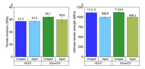
Figure 9: Tensile modulus (a) and ultimate tensile strength (b) properties obtained by longitudinal tensile test for both aged and unaged CF /  $Elium^{TM}$  and CF /  $Elium^{TM}$  CF / VE samples
