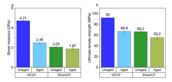
Figure 11: Shear modulus (a) and ultimate tensile strength (b) properties obtained by off-axis tensile test for both aged and unaged CF/VE and  $CF/Elium^{TM}$  specimens
