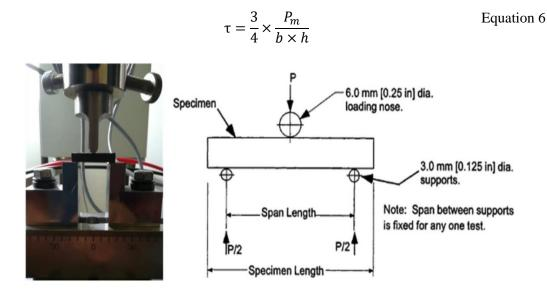
Figure 2: ILSS device (left) and test diagram (right) for rectangular laminates where:  $P_m$  is the maximum load observed during the test (N), b and h are the measured width and thickness (mm), respectively.
