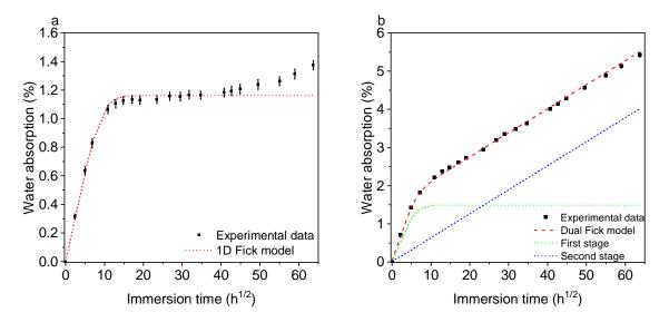
Figure 3: Experimental data and model results of water absorption as a function of the square root of the immersion time of (a) VE and (b) Elium<sup>TM</sup> resin specimens immersed in water at 70
