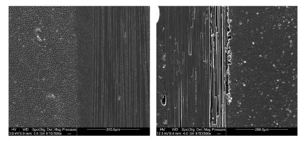
Figure 5 : SEM pictures of the microstructure of CF / VE (left) and CF / Elium $^{TM}$  composite (right) before aging
