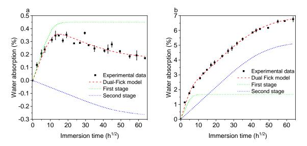
Figure 4: Evolution of water absorption as function of the square root of the immersion time of
