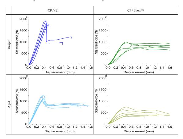
Figure 12: ILSS force-deformation curves of (a) unaged CF / VE specimens, (b) aged CF / VE specimens, (c) unaged CF / Elium<sup>TM</sup> specimens and (d) aged CF / Elium<sup>TM</sup> specimens
