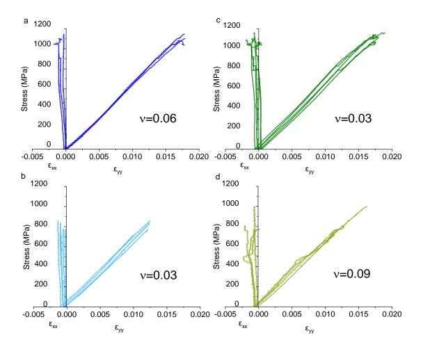
Figure 8: Tensile stress-strain curves of 0°/90° specimens: (a) unaged CF/VE specimens, (b) aged CF/VE specimens, (c) unaged CF/Elium<sup>TM</sup> specimens and (d) aged CF/Elium<sup>TM</sup> specimens
