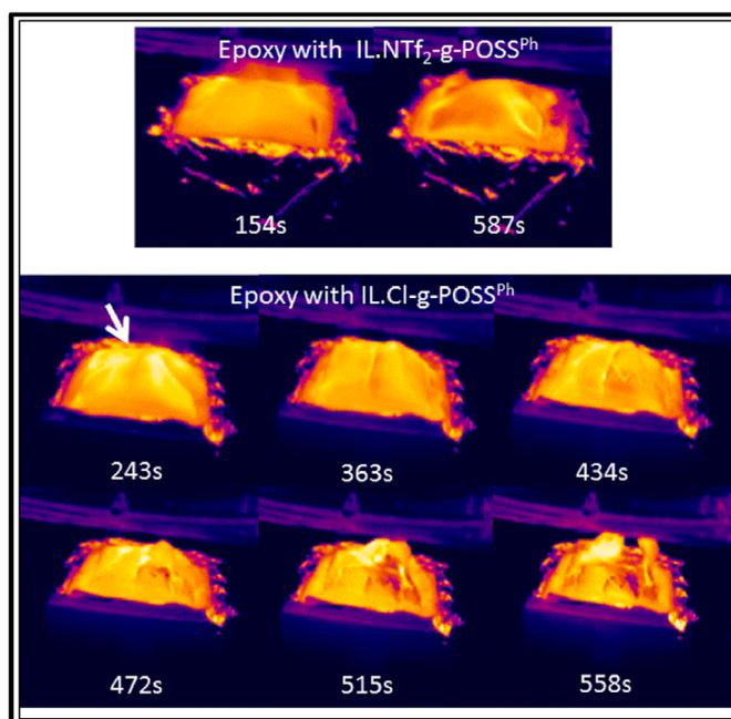
Fig. 9. Pictures obtained using thermal camera from cone calorimeter test of the hybrid O/I epoxy networks containing IL.NTf<sub>2</sub>-g-POSS<sup>Ph</sup> and IL.Cl-g-POSS<sup>Ph</sup>.
