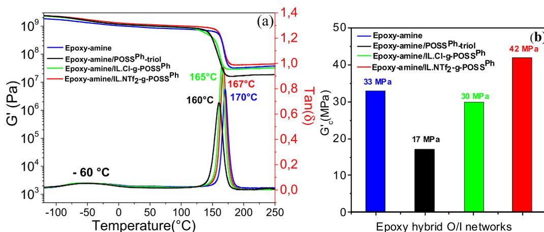
Fig. 4. a) Dynamic mechanical spectra and b) the shear storage moduli,  $G'_c$  (at 200 °C) of the epoxy-amine and the hybrid O/I epoxy networks containing POSS<sup>Ph</sup>-triol and IL-g-POSS<sup>Ph</sup> with different anions (Cl<sup>-</sup> and NTf<sub>2</sub>) at 1 Hz.
