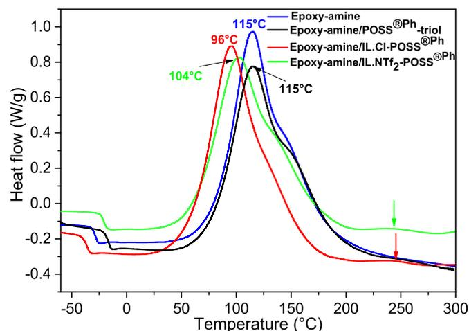
**Fig. 1.** DSC traces of neat epoxy-amine and the hybrid O/I epoxy reactive systems containing 5 wt % POSS<sup>Ph</sup>-triol or IL-g-POSS<sup>Ph</sup> with Cl<sup>-</sup> or NTf<sub>2</sub><sup>-</sup> anion (heating rate:  $10\text{ }^{\circ}\text{C min}^{-1}$ ).
