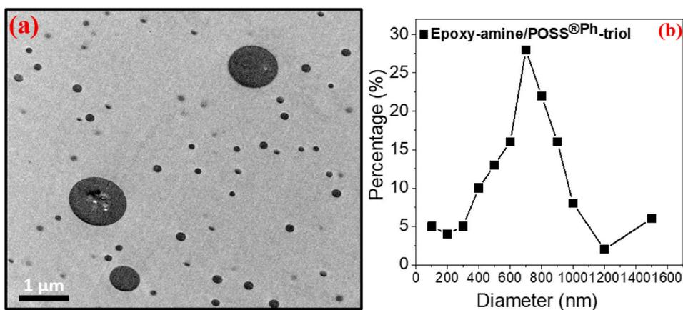
Fig. 2. a) TEM micrograph of the hybrid O/I epoxy network containing POSS<sup>Ph</sup>-triol, b) Size distribution of POSS<sup>Ph</sup>-triol aggregates.
