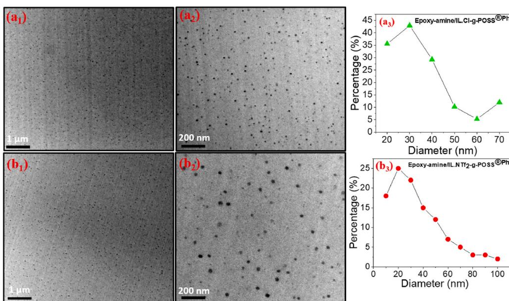
Fig. 3. TEM micrographs of the hybrid O/I epoxy networks containing: a) IL.Cl-g-POSS<sup>Ph</sup> at different magnification (a<sub>1</sub>; a<sub>2</sub>), b) IL.NTf<sub>2</sub>-g-POSS<sup>Ph</sup> at different magnification (b<sub>1</sub>; b<sub>2</sub>) and their size distribution (a<sub>3</sub>, b<sub>3</sub>).
