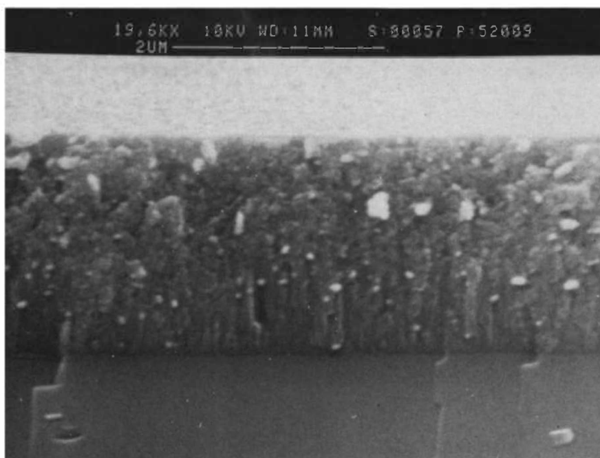
Fig. 8. Granular texture of amorphous \text{Al}_2\text{O}_3 and columnar texture of AlN, from 900°C to 1000°C.
