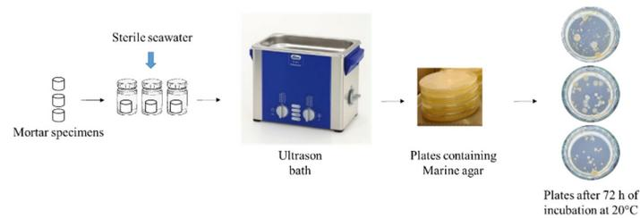
**Figure 6.** Culture-based method used in the quantification of bacterial biofilm formed on the surface of mortar specimens.
