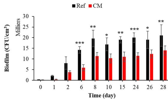
**Figure 14.** Quantification of bacterial biofilm on treated and untreated mortars with curing compound. Each experiment was performed in triplicate, and the error bars present the standard deviation of the values obtained. The experiments highlighted with asterisks differed significantly from the control (Bonferroni; \*:  $p < 0.05$ , \*\*:  $p < 0.01$ , \*\*\*:  $p < 0.001$ ) at the indicated time.
