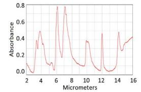
Figure 1: Typical hydrocarbons fire emission spectrum
