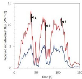
Figure 11: Incident heat flux from pool fire
