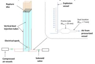
Figure 1: Sketch of the experimental setup
