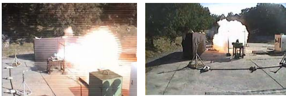
Figure 6: Ignition of LPG cloud
