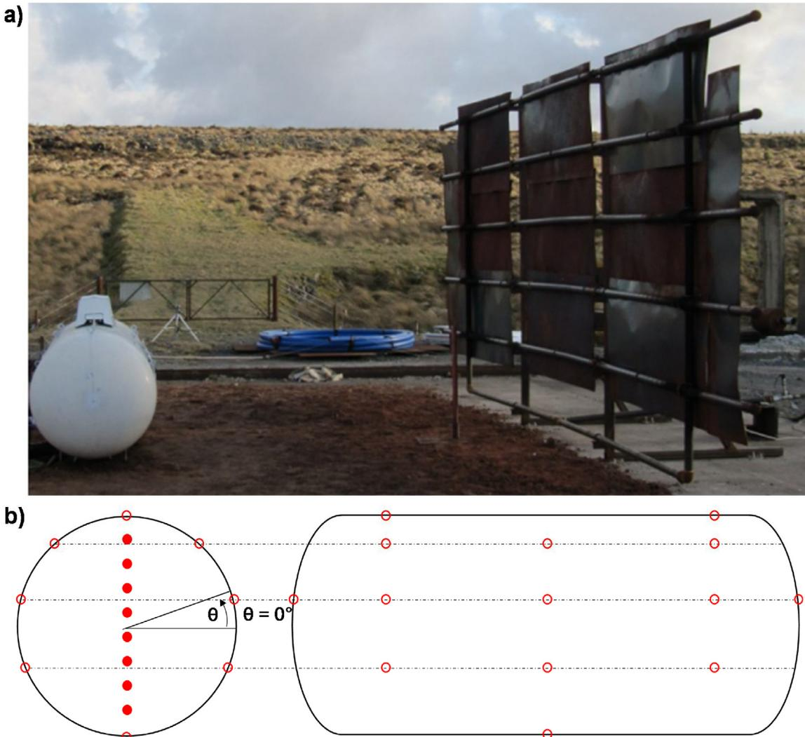
**Fig. 1 – Experimental apparatus configuration. a) The steel wall to reproduce the fire scenario is visible on the right; the tank is on the left. b) sketch of the thermocouples positioning in the lading (filled dots) and on the tank wall (empty dots).**
