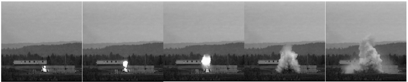
Fig. 1 – BLEVE of 1.9 m 3 propane tank, 50% full of liquid, failure pressure 2 MPa ( \Delta t between frames: 33 ms).
