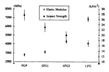
FIGURE 5 Results of impact and tensile test on powder, short and long fiberglass.
