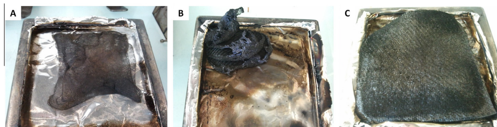
Fig. 16. Residues of (A) PES/F, (B) PES/F-MAPC1 and (C) PES/F-MVP composites after cone calorimeter test.
