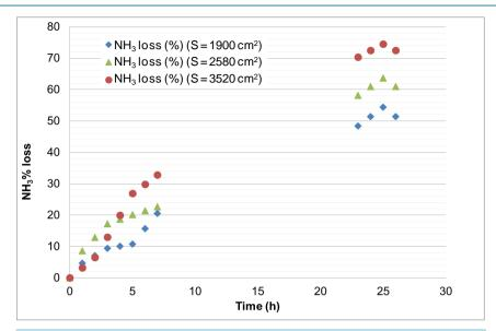
**Figure 6.** NH<sub>3</sub> loss (%) over time from the three bags having different surfaces (1900 cm<sup>2</sup>, 2580 cm<sup>2</sup> and 3520 cm<sup>2</sup>, respectively) and different S/V ratios (0.63 cm<sup>-1</sup>, 0.86 cm<sup>-1</sup> and 1.17 cm<sup>-1</sup>, respectively).
