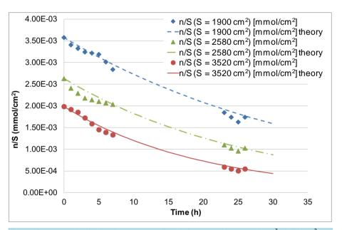
**Figure 5.** n/S trends for the three bags having different surfaces (1900 cm<sup>2</sup>, 2580 cm<sup>2</sup> and 3520 cm<sup>2</sup>, respectively) and different S/V ratios (0.63 cm<sup>-1</sup>, 0.86 cm<sup>-1</sup> and 1.17 cm<sup>-1</sup>, respectively).
