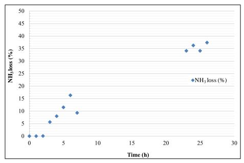
Figure 3. NH<sub>3</sub> loss (%) over time from the Nalophan<sup>TM</sup> bag with  $V_N = 6000 \text{ cm}^3$  and  $S_N = 2580 \text{ cm}^2$ .
