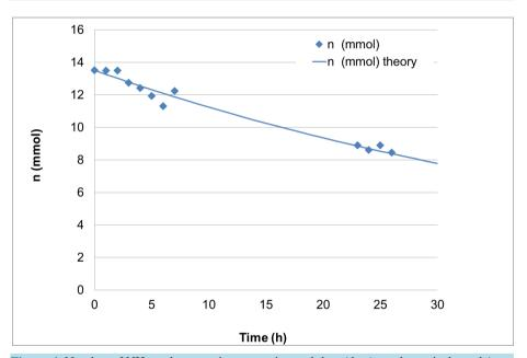
Figure 4. Number of NH<sub>3</sub> moles over time: experimental data (dots) vs. theoretical trend (continuous line) in a Nalophan<sup>TM</sup> bag with  $V_N = 6000 \text{ cm}^3$  and  $S_N = 2580 \text{ cm}^2$ .
