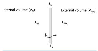
Figure 2. Schematization of diffusion through the thin film of the bag.
