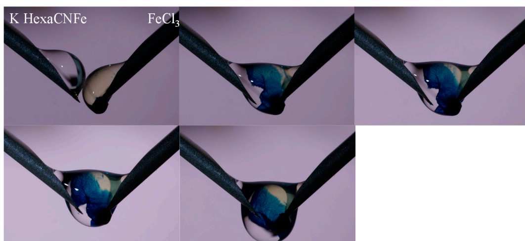
Figure 1. “In-drop” synthesis of Prussian Blue.
