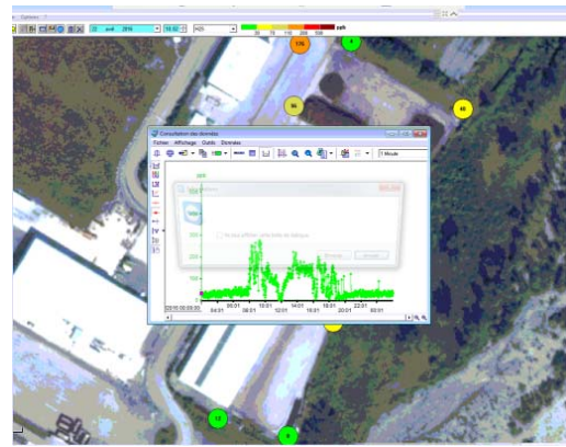
Figure 5: (a) H_2S sensor measurements on the site, (b) An example of H_2S sensor measurements along one day
