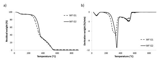
Fig. 5. Residual weight (a) and derivative weight (b) of WF G1 and WF G2 by TGA under an air atmosphere.
