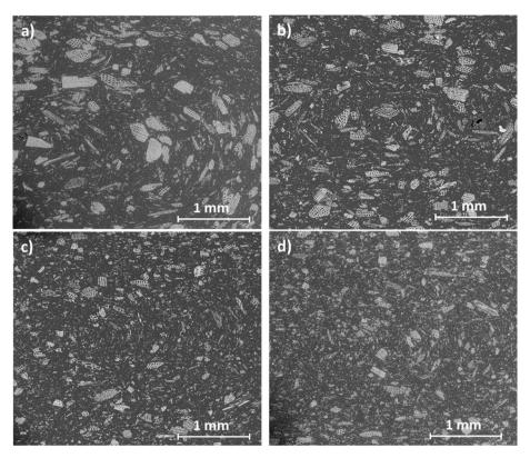
Fig. 15. SEM micrographs of transversal cross sections of PP/PPgma/WF G2 at P1 (a), P3 (b), P5 (c) and P7 (d) (magnification ×80).
