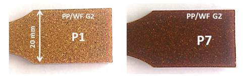
Fig. 13. Surface color change of PP/WF G2 from P1 to P7.
