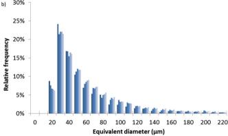
**Fig. 11.** Comparison of relative frequency by number of the particle equivalent diameter of WF G1 (a) and WF G2 (b) as a function of processing cycles from the initial state (darker color) to P7 (lighter color).(For interpretation of the references to colour in this figure legend, the reader is referred to the web version of this article.)
