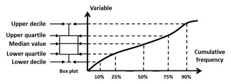
Fig. 4. A schematic presentation of the box plot method based on the cumulative distribution function of an experimental data set.
