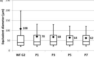
**Fig. 10.** Box-plot representation and average (square dots) of the equivalent diameter of WF G1 (a) and WF G2 (b) as a function of processing cycles.
