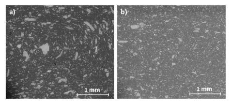
Fig. 8. SEM micrographs of transversal cross sections of PP/WF G1 at P1 (a) and at P7 (b) (magnification ×80).
