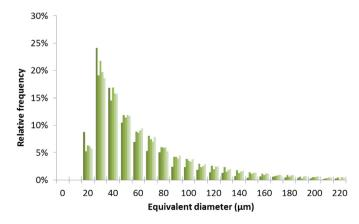
**Fig. 17.** Relative frequency by number of the particle equivalent diameter of WF G2 in the PP/PPgma/WF composite as a function of processing cycles from the initial state (darker color) to P7 (lighter color).(For interpretation of the references to colour in this figure legend, the reader is referred to the web version of this article.)
