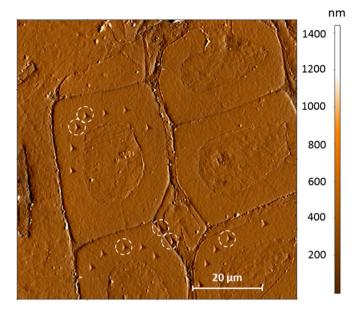
Fig. 3. AFM cartography of indented surface of the PP/WF G2 composite.
