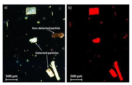
Fig. 2. Microscopic picture of wood flour particles under polarized light before (a) and after (b) image thresholding by Aphelion of software.
