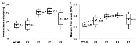
Fig. 18. Box plot representation and average (square dots) of nanoindentation characteristics of wood cell walls: indentation modulus (a) and indentation hardness (b) of WF G2 in the PP/PPgma/WF composite through the processing cycles.
