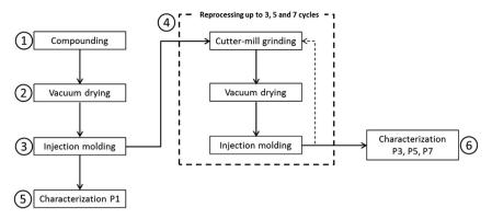
Fig. 1. Stages of the processing method by grinding and injection.
