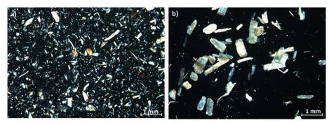
Fig. 6. Microscopic observations with a crossed polarized light of the two types of wood flour: WF G1 (a) and WF G2 (b) (magnification ×10).
