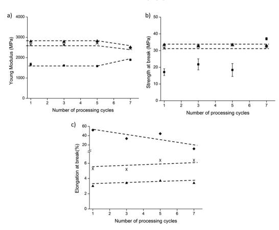
**Fig. 14.** Young modulus (a), strength at break (b) and elongation at break (c) measured by tensile test at 1, 3, 5 and 7 processing cycles *of neat PP* (■), *PP/WF G1* (X) and *PP/WF G2*(▲).
