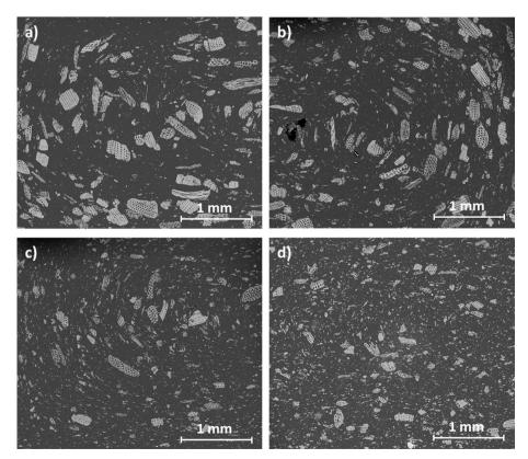
Fig. 9. SEM micrographs of transversal cross sections of PP/WF G2 at P1 (a), P3 (b), P5 (c) and P7 (d) (magnification ×80).
