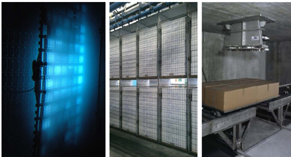
Fig. 11. Pictures of industrial facilities: (left) Gamma radiation source and (middle) several containers of a full conveyor at Ionisos facility in Dagneux (France); (right) radiation treatment of a pallet layer at Ionisos facility in Tarancon (Spain). Copyright (2017) Ionisos SAS.
