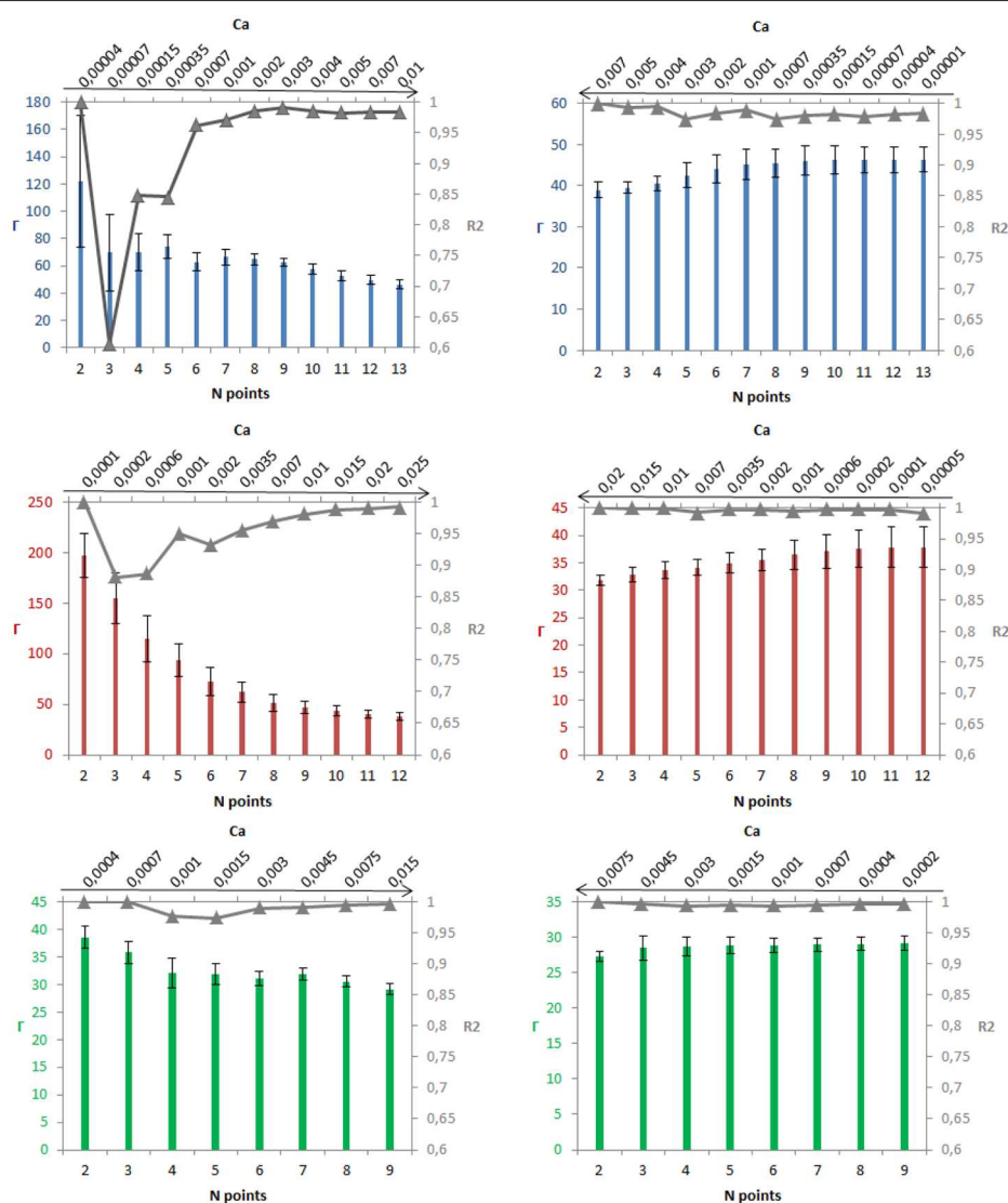
FIGURE 7 | Sensitivity of \Gamma for PEG1450 (blue), PEG3350 (red), and PEG10000 (green): from the lowest Ca to the highest one (left); from the highest Ca to the lowest one (right).
