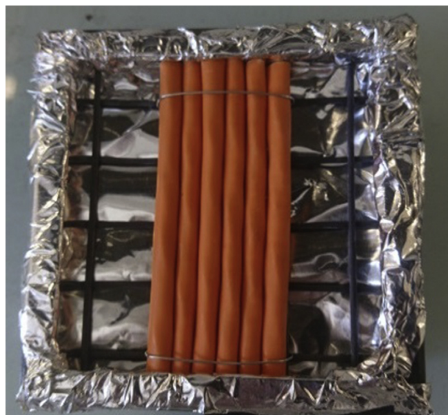
Fig. 3. Samples of cables attached to a grid – aluminium folder is placed between the grid and the sample holder.
