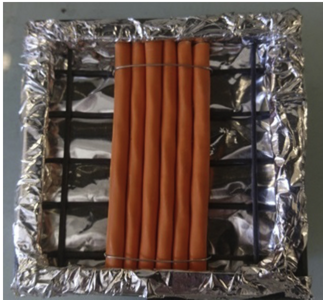
Fig. 3. Samples of cables attached to a grid – aluminium folder is placed between the grid and the sample holder.
