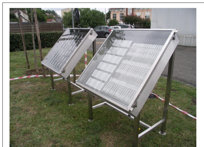
FIGURE 1 | Under windshield glass exposure racks.
