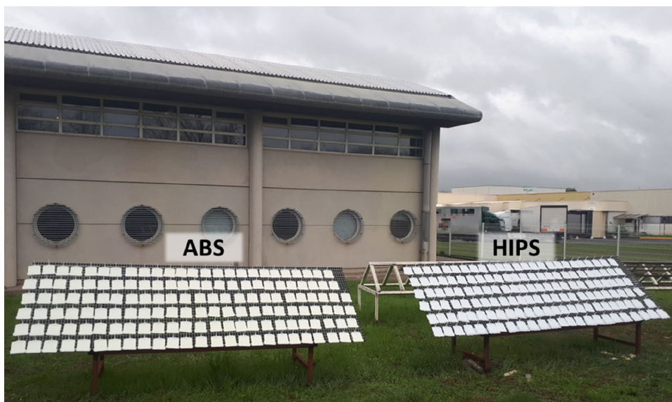
Fig. 3 Polymer plates put to natural ageing on metallic racks in Alès, France (44° 08' 09.0" N 4°05'54.3"E)
