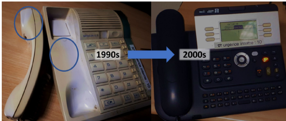
Fig. 1 Example of black coloration generalization for small WEEE plastics—note tint difference between exposed and preserved areas of the 1990s phone station
