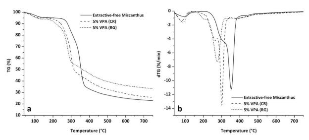
Fig. 6. TGA (a) and dTG (b) curves for miscanthus fibers, miscanthus fibers modified by condensation reaction (CR) under mild conditions and by radiografting (RG) at 50 kGy with a 5 wt% VPA solution.
