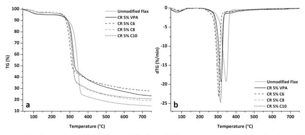
Fig. 11. TGA (a) and dTG (b) curves for unmodified flax fibers and for flax fibers modified by condensation reaction (CR) under mild conditions with a 5 wt% solution of VPA, C6, C8 or C10.
