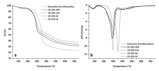
Fig. 9. TGA (a) and dTG (b) curves for miscanthus fibers and for miscanthus fibers modified by condensation reaction (CR) under mild conditions with a 10 wt% solution of VPA. C10. C8 or C6.
