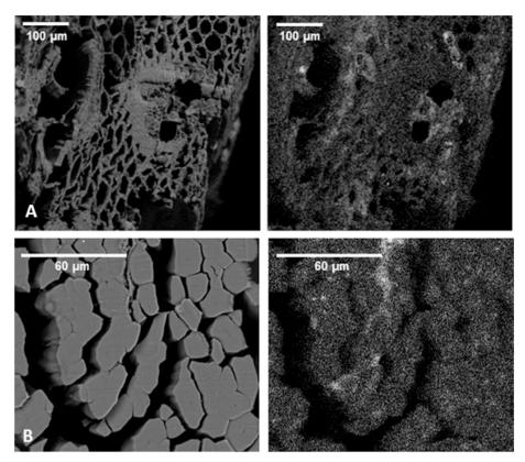
Fig. 4. SEM images (left) and EDX phosphorus mapping (right) of miscanthus fibers (A) and flax fibers (B) treated with solutions of 5 wt% C6 bisphosphonic acid aqueous solutions by chemical modification under mild conditions
