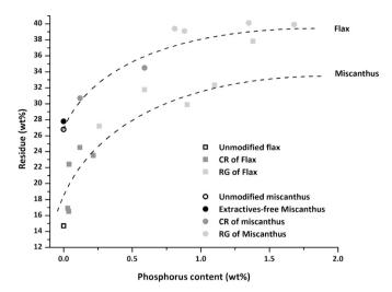
Fig. 17. Variation of residue percentage at 750  $^{\circ}$ C (anaerobic degradation - TGA) as a function of phosphorus content for miscanthus and flax fibers modified by condensation reaction (CR) and radiation grafting (RG) with VPA.
