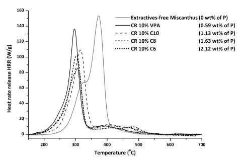
Fig. 8. HRR curves for miscanthus fibers and for miscanthus fibers modified by condensation reaction (CR) under mild conditions with a 10 wt% solution of VPA, C10, C8 or C6.
