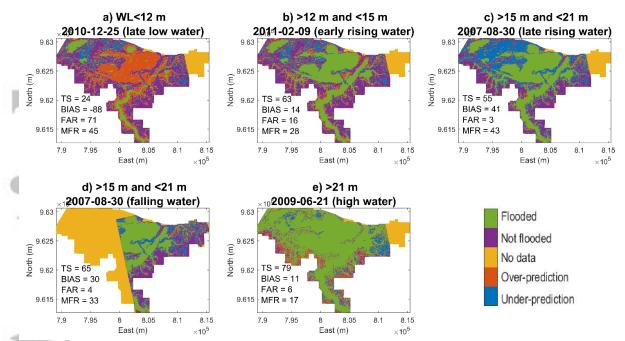
Figure 5. Comparisons of inundation extent obtained by TELEMAC-2D simulation against inundation maps for different periods a) WL<12 m (low water), b) 12 m WL<15 m (early rising water), c) 15 m <WL<21 m (late rising water) d) 15 m <WL<21 m (falling water), e) WL>21 m (high water)
