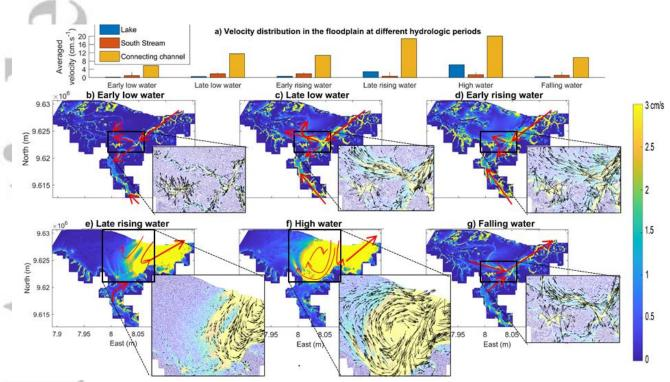
Figure 7. a) Average velocity distribution following the hydrologic period, b)-g) velocity distribution in the FP at different hydrological periods with velocity magnitude in cm.s<sup>-1</sup> set as background. The schematic red and black arrows indicate the direction of water circulation.
