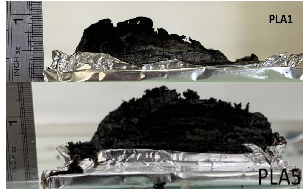
Fig. 12 : Cone calorimetry residue (PLA1 and PLA5)
