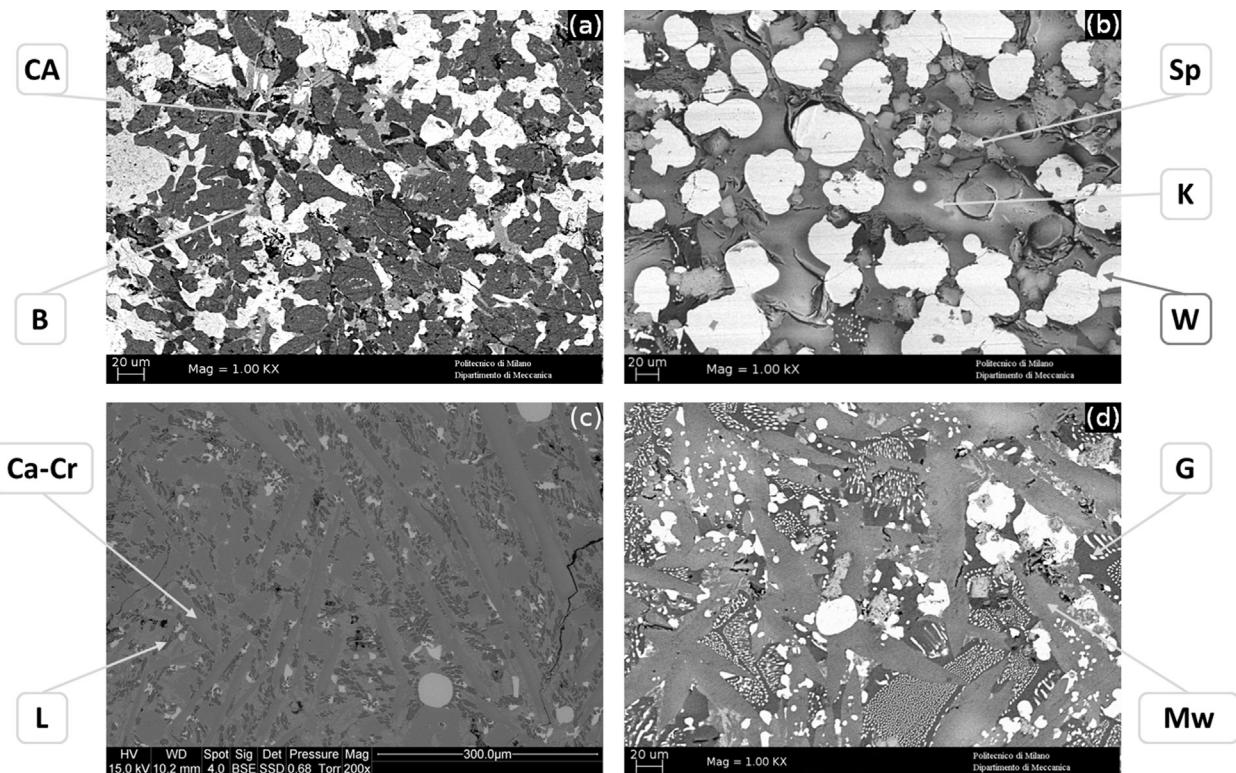
**Fig. 2 – Examples of microstructure: (a) sample #2; (b) sample #7; (c) sample #8 and (d) sample #12.** Refer to [Table 3](#) for abbreviations and formula.
