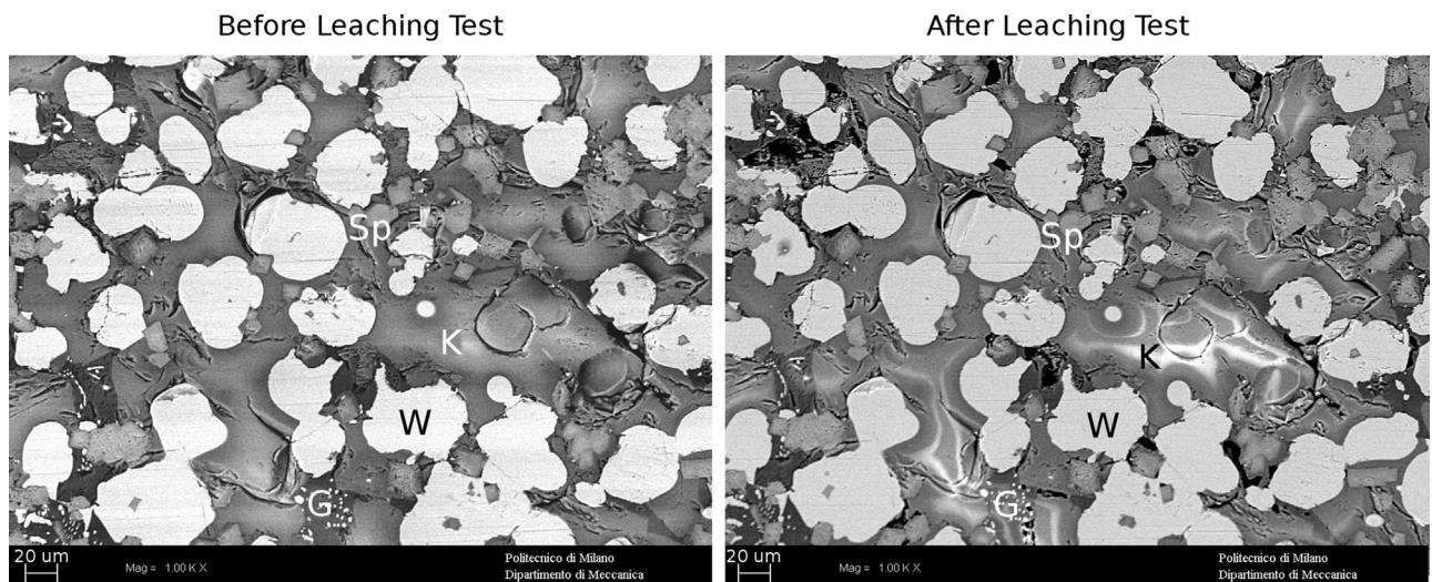
**Fig. 12 – SEM-BSE microographies of polished section before and after leaching test.**
