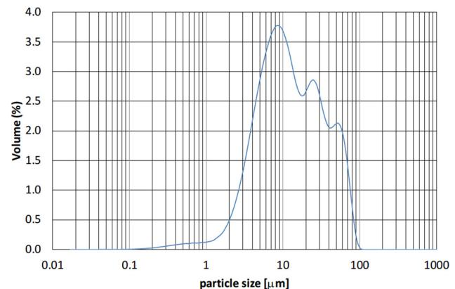
**Fig. 1 – Particle size distribution of investigated slag powder.**
