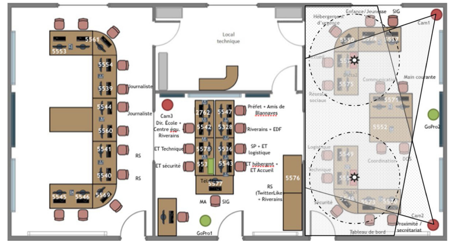
Fig. 1. Experimental installation with video cameras (red circles with field of view) and audio-recorders (black stars with approximate range). (Color figure online)
