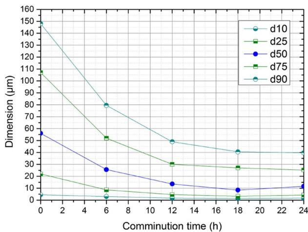
**Fig. 19** Particle size distribution measured by laser diffraction of PMC comminuted in a ball mill during different times (second ball set milling time)
