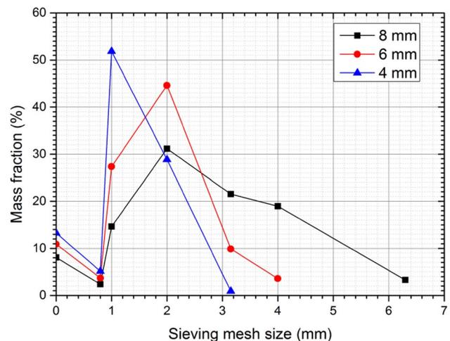
Fig. 11 Mass PSD of PMC crushed with a knife mill with 3 sizes of grid, measured by sieving (1500 rpm)
